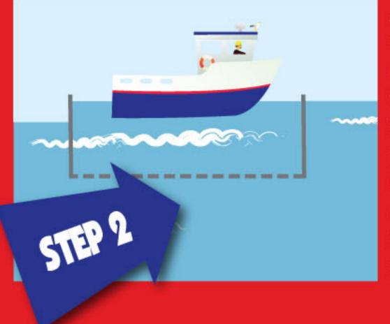
A valve is opened to allow water to flow into the lock (to raise the ship) or out of the lock (to lower the ship).
